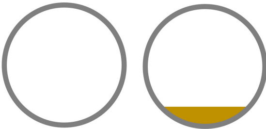
Figure 26. A pipe with and without sediments
