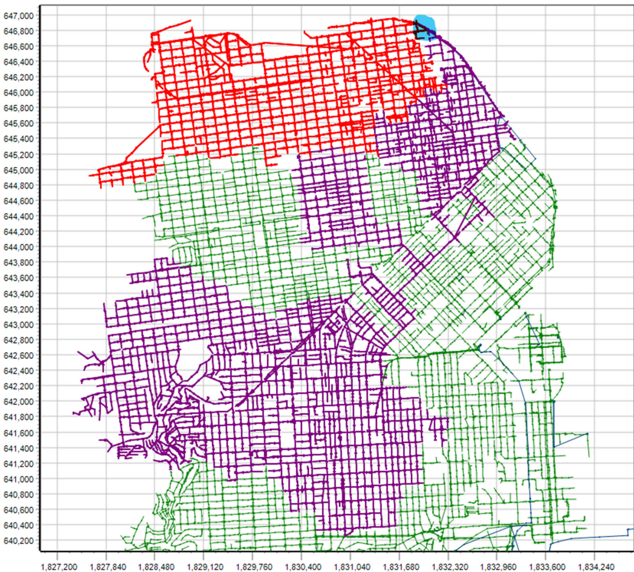
Figure 93. Two sub-catchments feeding a major pump station
