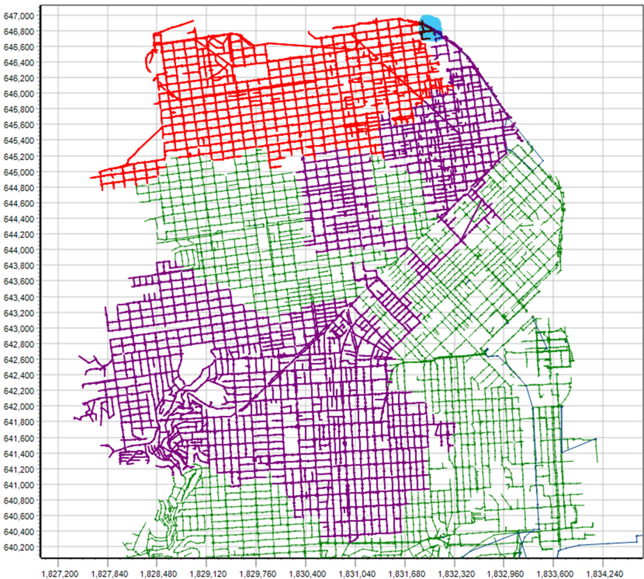
Figure 93. Two sub-catchments feeding a major pump station
