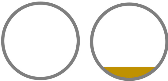
Figure 26. A pipe with and without sediments
